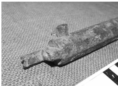
Figure 2: Breech of rifle barrel showing the tang, powder drum and nipple.
