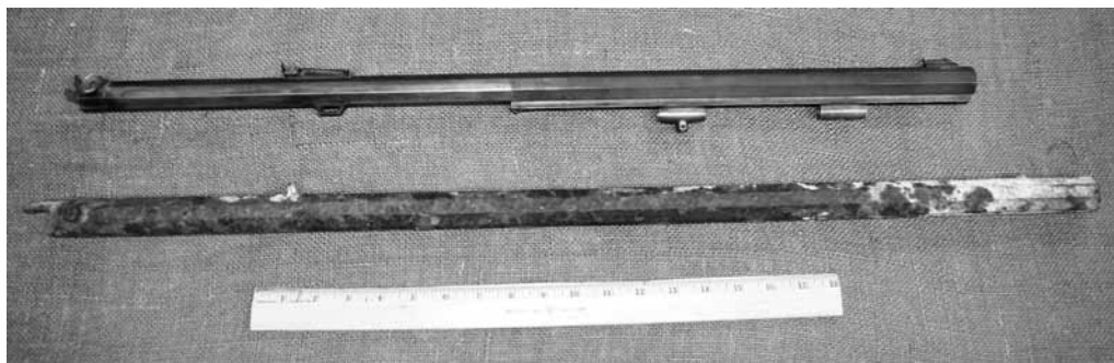
Figure 1: Modern T/C Hawken half-stock rifle barrel on top. The lower barrel is an historic caplock conversion with fixed dove tail and blade sights and a tang (wedge mount missing) which held it to the stock.
